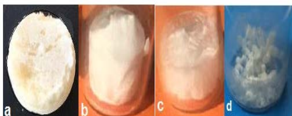
Fig. 1: Appearance of lyophilized matrix of intravesical BCG samples a)final sample with combination of lactose, MSG and tween 80, b) dextran-40 10%, c)sucrose 10% and MSG 10%.
