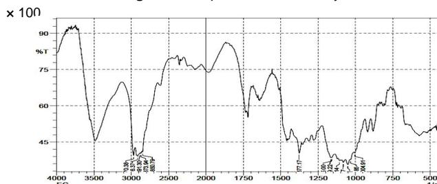
Figure-2: IR spectrum of Ethyl cellulose
