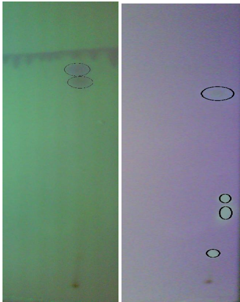
(a) TLC at 254 nm (b) TLC at 365 nm
