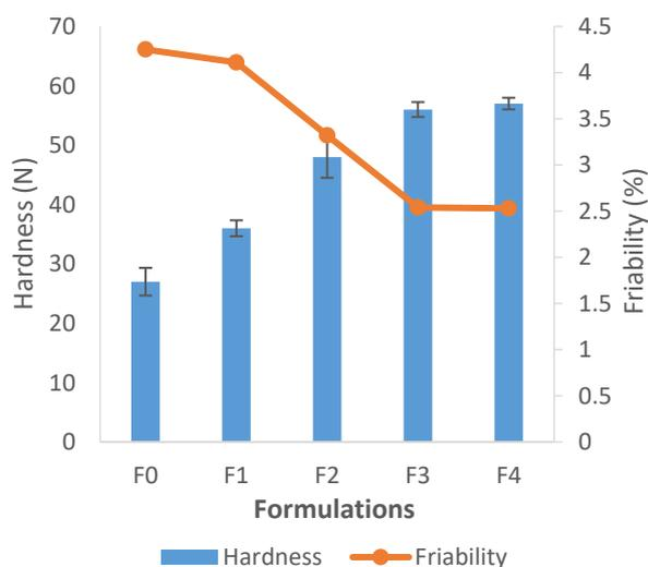
**Figure 4: Hardness and friability profile of control (F0) and milled metformin (F1-F4) tablets. Tablets were compressed at 3 tonnes compression force. Results of hardness were reported as mean±SD (n=3).**
