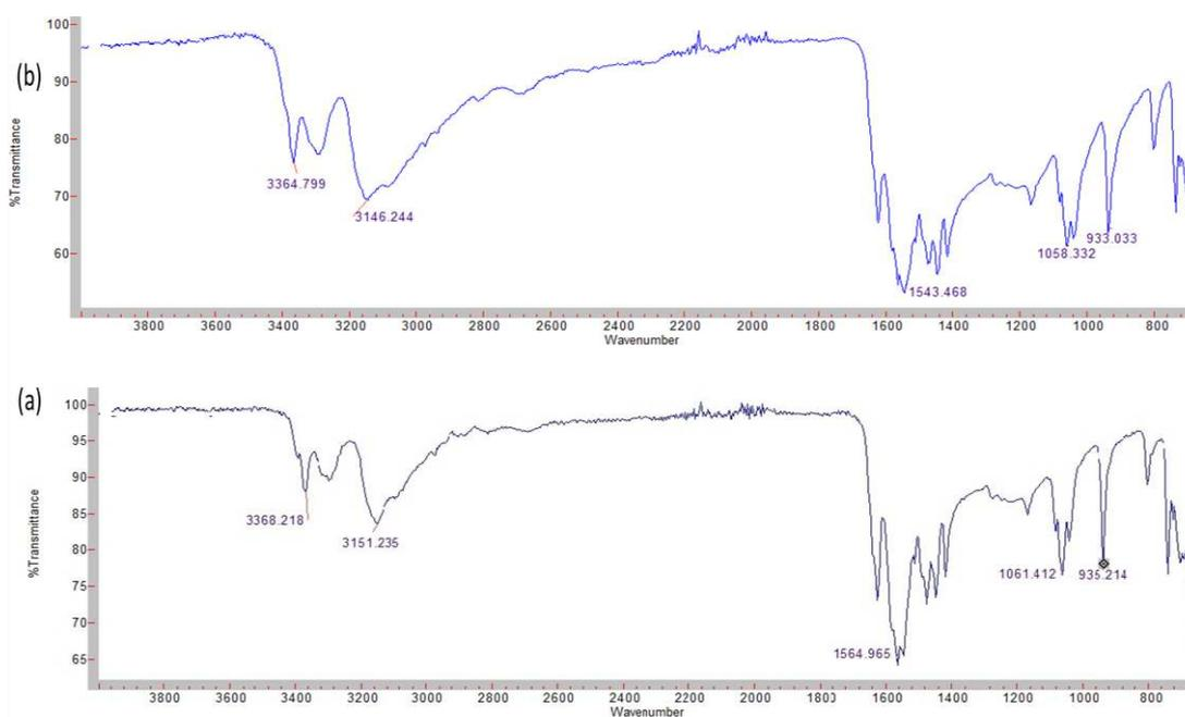
**Figure 3: FTIR spectra of (a) unmilled powder metformin HCL and (b) milled metformin (F4).**
