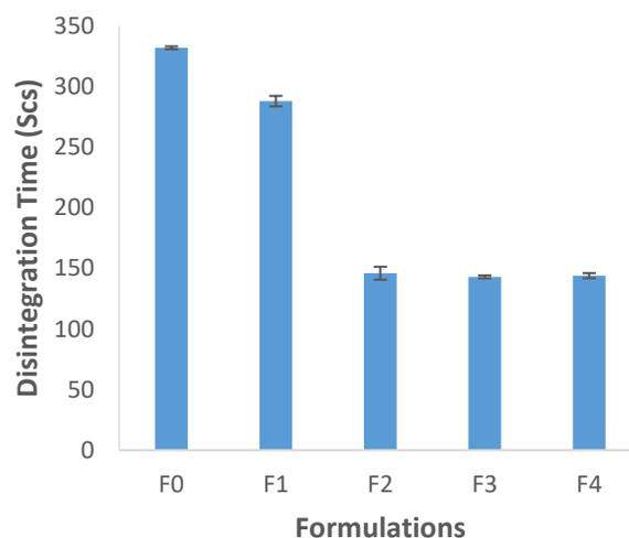
**Figure 5: Disintegration time profile of control (F0) and milled metformin (F1-F4) tablets. Tablets were compressed at 3 tonnes compression force. Results were reported as mean±SD (n=3).**
