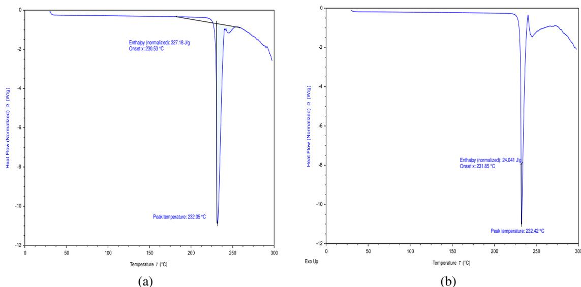
**Figure 2: DSC heating curves showing the melting point event as a function of temperature for (a) unmilled metformin powder (F0) and (b) milled metformin HCL (F4).**
