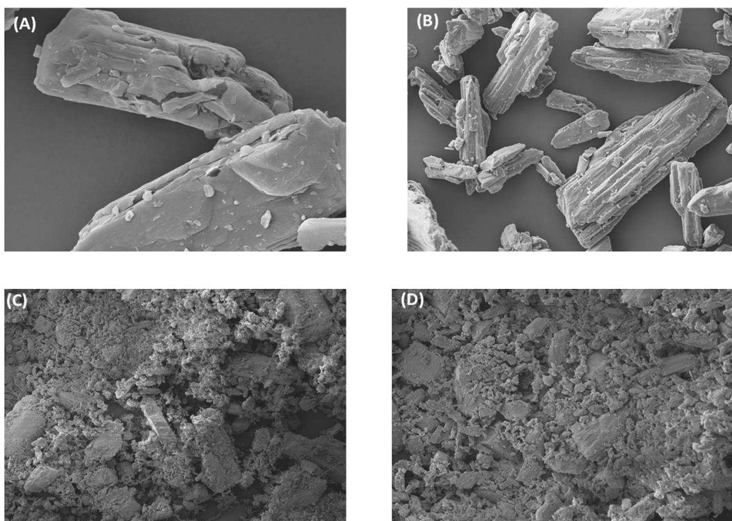
Figure 1: Scanning electron micrograph with different magnifications of (a and b) un-milled metformin HCL, and (c and d) milled metformin HCL (F4) powders.
