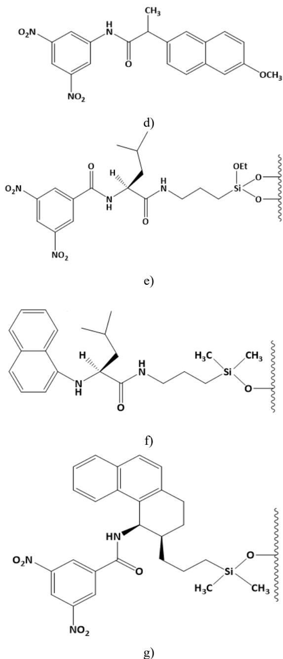
**Figure 1.** Pirklé type ( $\pi$ -donor– $\pi$ -acceptor) compounds (a, b, c, and d) and CSPs (e, f, and g)
